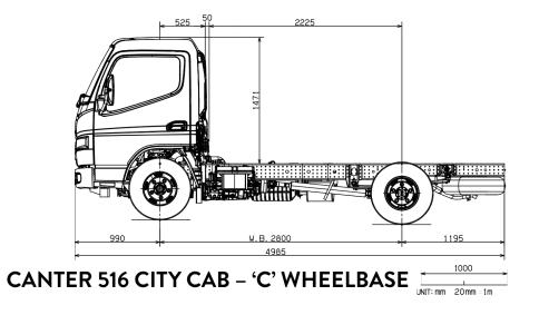
Scale = 1:50 (20mm = 1 metre). This scale is accurate when used on the original spec sheet, be aware that enlarging these illustrations can alter the scale and cause incorrect measurements. Fuso New Zealand and its authorised dealers always recommend customers seek professional advice from independent sources before commencing any engineering activities.
